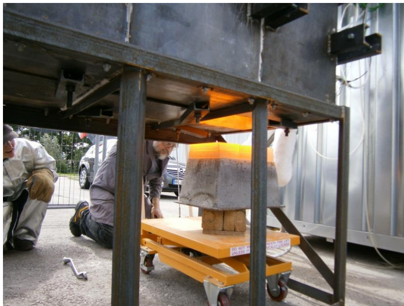
Figure 6: A crucible containing a glass batch sample is inserted into the test rig
