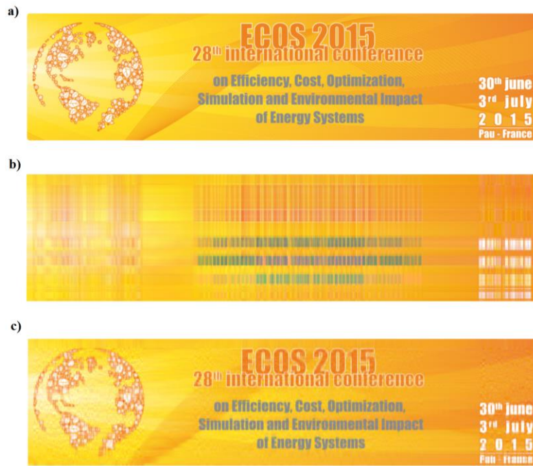
Fig. 1. Image reduction (i.e. compression) by POD. a) original image, b) contains 3% of original image, c) contains 10% of information of the original image.
