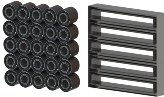
Fig. 2. A schematic of the concentric tube and heat exchanger with the thermoelectric junctions coupled.
