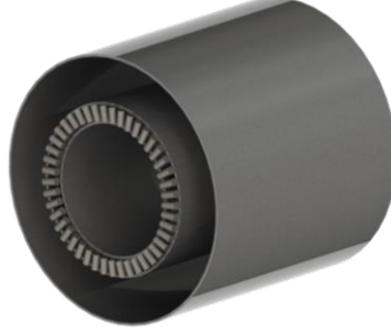
Fig. 3. A schematic of the concentric tube heat exchanger's module with the TEGs.
