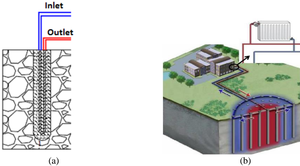
Fig. 1. BTES system: a) the vertical single U-Tube borehole and b) the direct connection with radiators.
